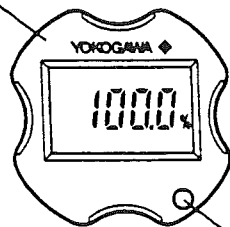
Figure 7.6 Range-setting Switch
